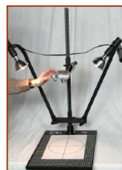
Light Stand with camera and template for hands and feet.
